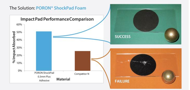
As you can see in the graph above, **PORON ShockPad Foam absorbs twice as much force as equivalent competitive material** in real-life drop conditions.
