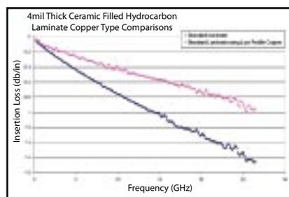
**Fig 5 A Ceramic Filled Hydrocarbon Laminate Compared to the Same Laminate Using a Low Profile Copper and Showing Insertion Loss Over Frequency<sup>2</sup>**
