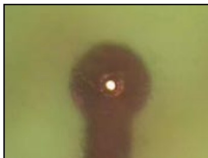
Fig 6 50µm (top) and 25µm (bottom) Blind Via Demonstrated in the Build-Up Material 2
