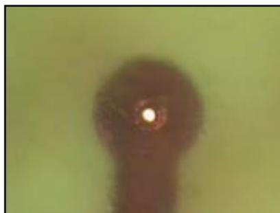
**Fig 6 50µm (top) and 25µm (bottom) Blind Via Demonstrated in the Build-Up Material<sup>2</sup>**
