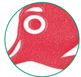
Soft PE tape print quality after 28,400 impressions with no adjustments.
