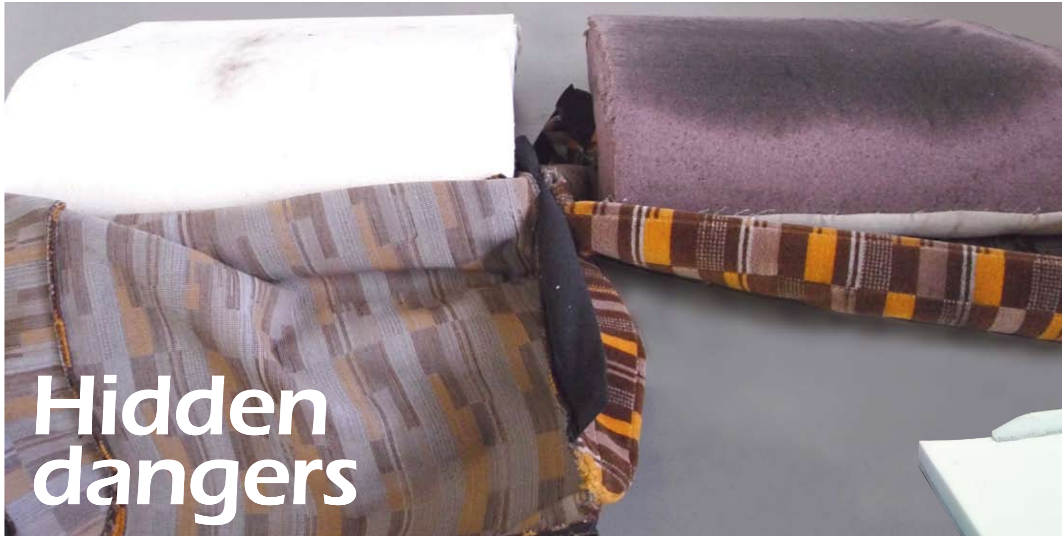
ABOVE LEFT: The impact of a 100,000-cycle test on silicone (left) and polyurethane (right) foam
