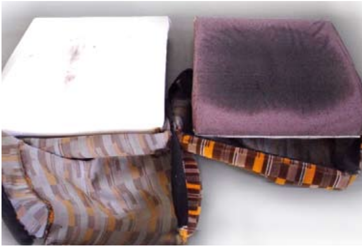
ABOVE: After a 100,000-cycle test, the silicone foam (on the left) remains largely unchanged
