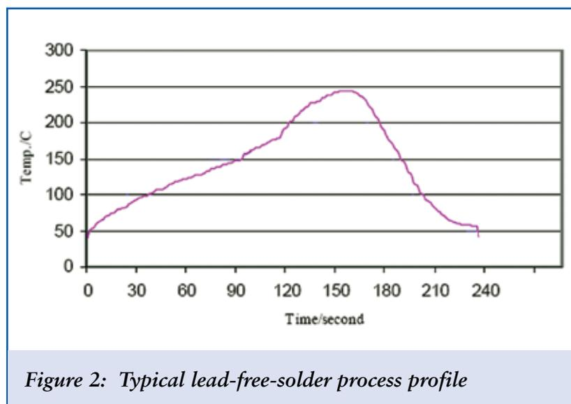
**Figure 2:** Typical lead-free-solder process profile
