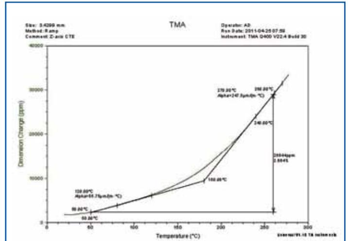
Figure 3: TMA curve for a thermoset PCB material
