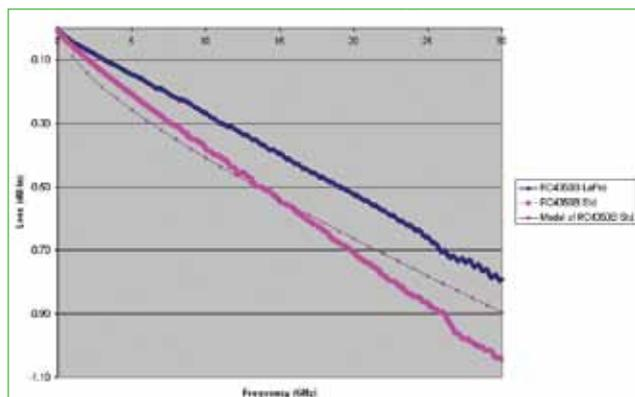
**FIGURE 3.** Insertion-loss responses for identical 0.010" microstrip circuits fabricated on a standard RO4350B laminate with normal copper conductor surface roughness and RO4350B LoPro laminate. The third response was generated by Rogers' MWI-2010 Microwave Impedance Calculator, which uses the Morgan rule to account for conductor surface roughness.
