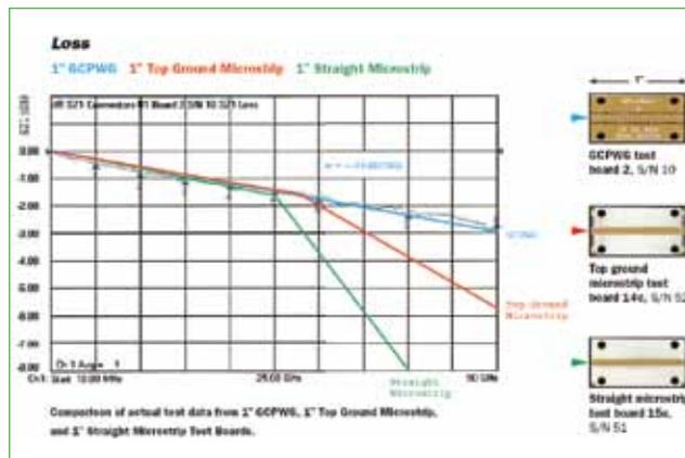
**FIGURE 6.** A study<sup>3</sup> revealed differences among conventional microstrip, microstrip with a top ground launch or coplanar launch, and CBCPW (referred to as GCPWG in the study) transmission lines.
