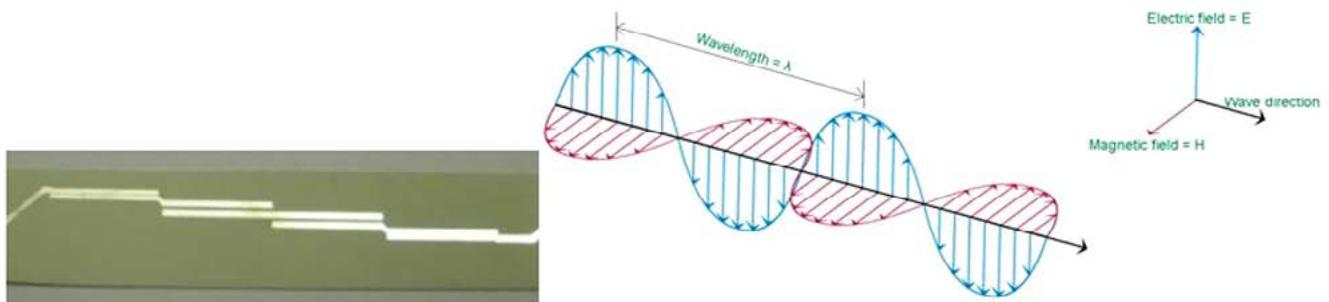
Figure 1. Microstrip edge-coupled bandpass filter as part of the PCB pattern, and a wavelength illustration.
