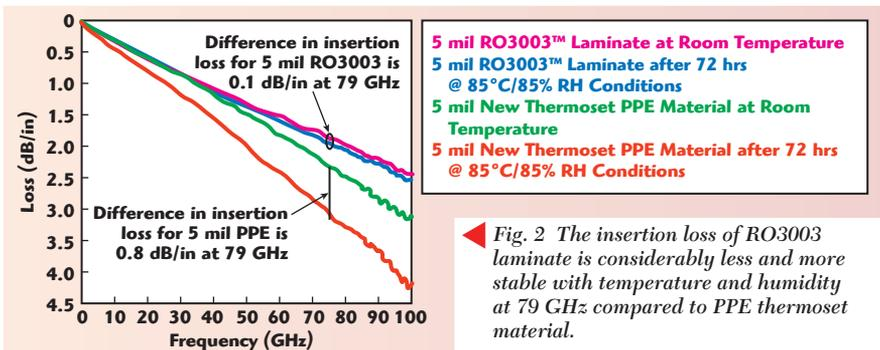
◀ Fig. 2 The insertion loss of RO3003 laminate is considerably less and more stable with temperature and humidity at 79 GHz compared to PPE thermoset material.
