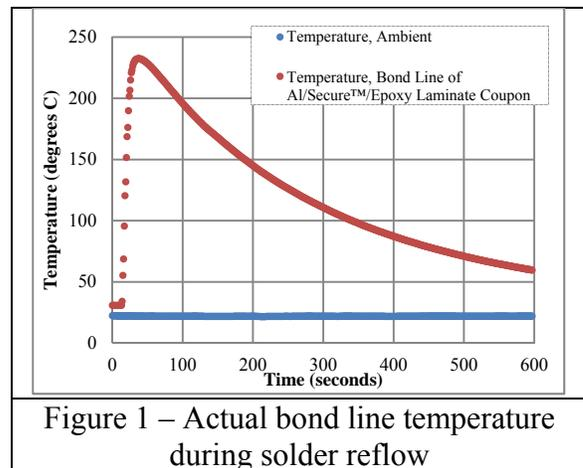
rise possible and the greatest thermal shock. This method produced an initial temperature rise of 1,022°C per minute.
