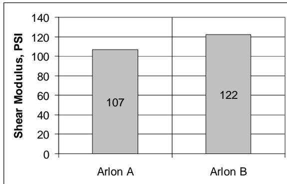
Figure 6 – Shear modulus of Arlon A and B
