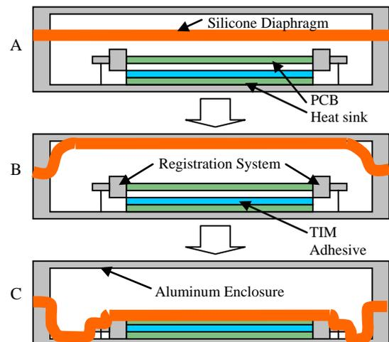
**Figure 3 – Schematic of the DVPL lamination process. (A) Atmospheric pressure in both chamber of DVPL with the PCB separated from the adhesive by the registration system. (B) Vacuum drawn in top chamber of DVPL. (C) Vacuum drawn in bottom chamber and top chamber vented to atmosphere. Silicone diaphragm has descended, mated the PCB to the adhesive, and is applying pressure to the assembly.**
