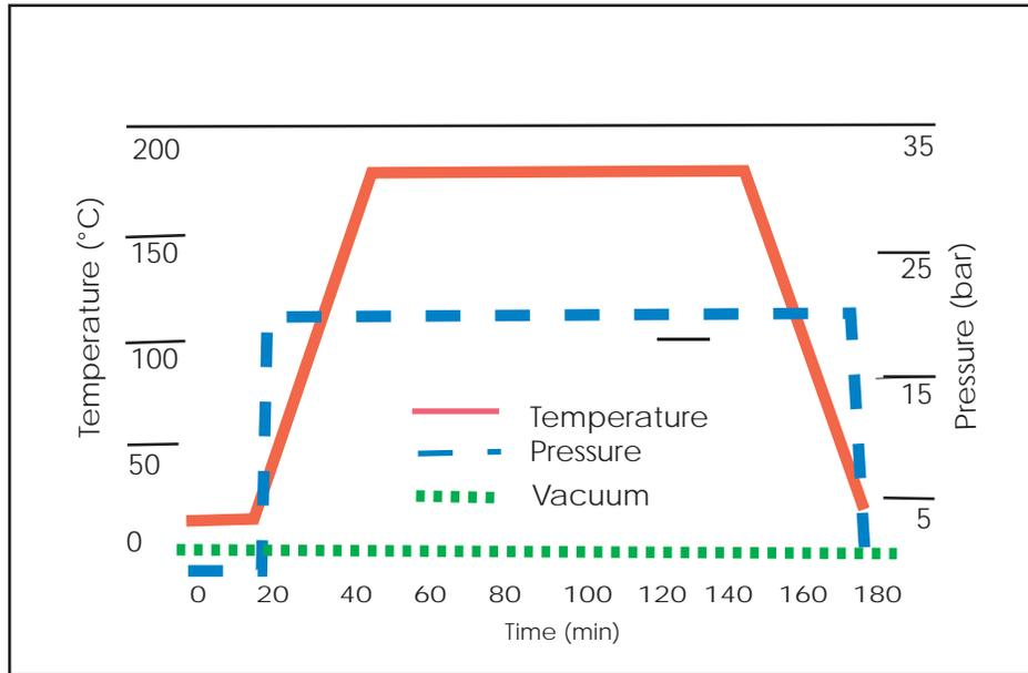
The high temperature requirement for direct bonding requires exclusion of air to avoid copper oxidation that destroys the bond of copper to base material. Air also causes degradation of the PTFE evident as a whitened or bleached appearance and may increase dissipation factor.
