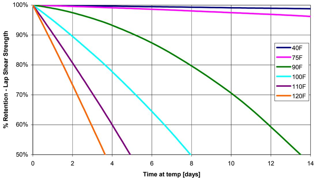
**Figure 2 - Primerless Thermabond® stability at temperature (0 - 14 days)**
