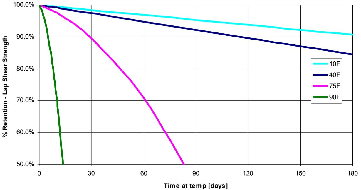
**Figure 1 - Primerless Thermabond® stability at temperature (0 - 180 days)**
