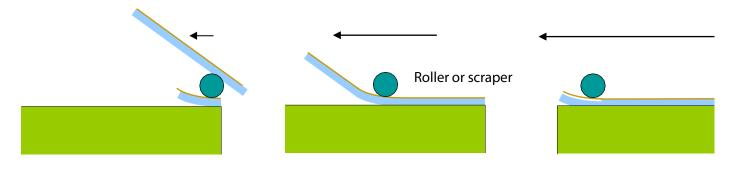
3. Remove brown PTFE-coated fiberglass substrate
