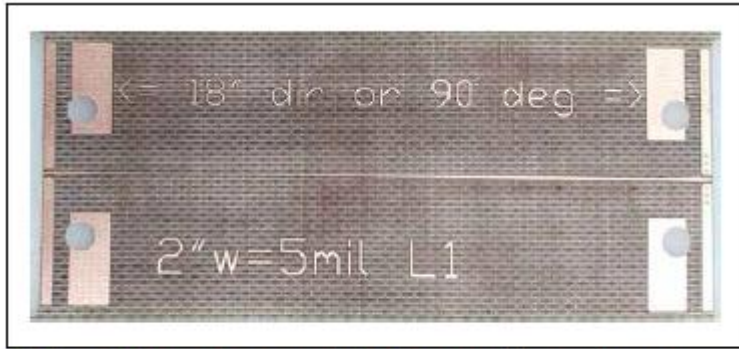
▲ Fig. 3 Microstrip transmission line transitioning from a GCPW.
