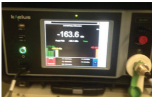
Figure 2. A high-performance test set with PIM analyzer provides measurement results on the PIM levels from different circuit laminates.
