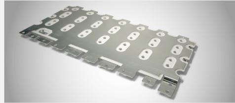
**ROLINX Easy** laminated busbars eliminate the outer insulation. They utilize a closed mold technology which offers high short circuit resistance, optimized inductivity and high currents above 1000A. Ideal for low and medium voltage applications.
