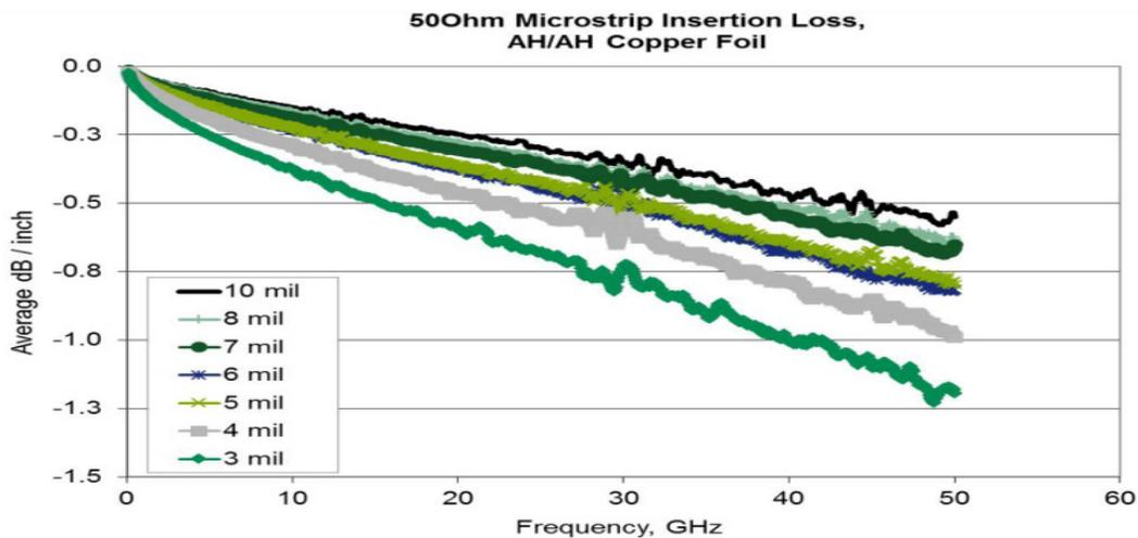
Figure 3. 50 Ohm Microstrip Insertion Loss
