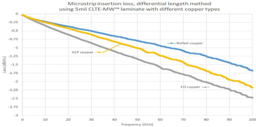
Figure 2. Microstrip Insertion Loss, Differential Length Method
