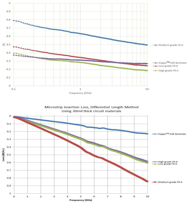
Microstrip differential phase length method, Dk vs. Frequency using 30mil thick circuit materials
