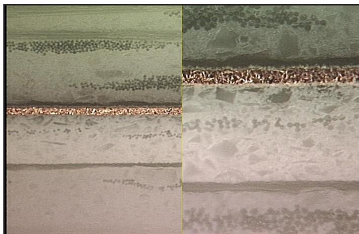
*Visual comparison of RO4000 LoPro laminates and traditional RO4000 cores in multi-layer constructions.*
