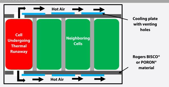
Vent paths are created in battery packs to direct the hot air from a cell undergoing thermal runaway away from the neighboring cells and out of the cell pack. A Rogers material can help guide hot air through a vent when it bursts at high temperatures, allowing heat to escape while keeping the area between the cooling plate and cell spacer sealed to prevent a full thermal runaway.
