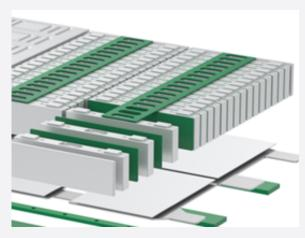
Some battery pack manufacturers have designed air ducts to direct the hot gasses out and away from the other lithium-ion cells into the designed vent path. To ensure the hot air is dispersed through the ducts they need a gasket seal between the duct and the battery racks. BISCO® materials are compressible and capable of withstanding extreme heat for short durations to ensure the hot gasses proceed down the design path for maximum safety of the pack and passengers.
