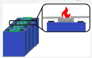
At the cell level, vent channel gaskets are often used with prismatic form factor because they have a factory vent. A foam gasket can be used around the cell vent to divert hot gas and ejecta away from neighboring cells. Vent channels can be used at the pack or module level of any form factor to direct hot gas and ejecta away from critical components or direct gas towards sensors for earlier detection of a thermal event.
