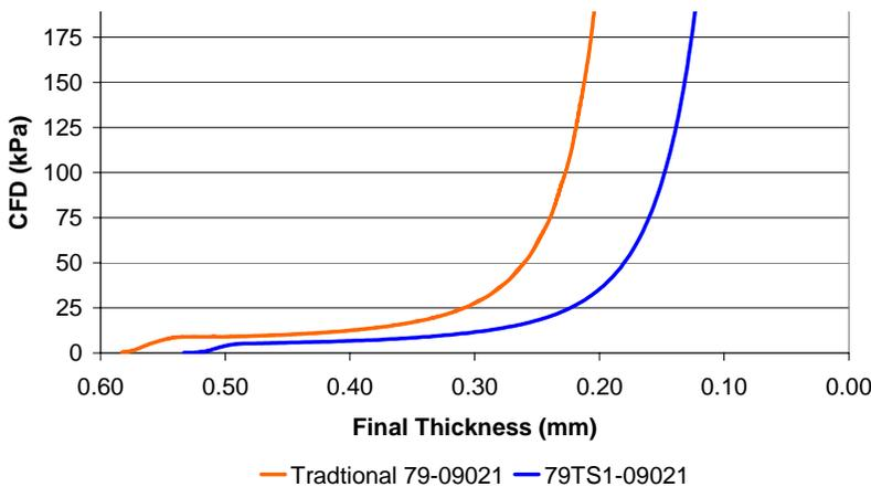
79TS1 exhibits all the reliable features PORON Foams are known for, and within the ShockSeal series of foams, is the most compressible. This added compressibility is an inherent benefit of working within the ThinStik family.
