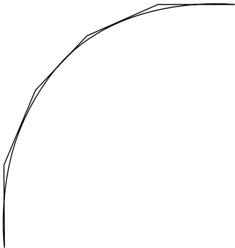
*Figure 5: Straight Cuts in place of fabricated Radii*
