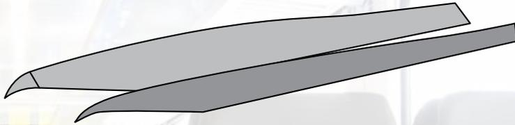
**Bottom Pad:** Often referred to as the actual seat cushion or a support for a main cushion. This component may be part of a full seat assembly or a simple pad that is part of an ergonomically designed seat pan.
