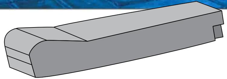
**Seat Back:** The portion of a seat design that may or may not be padded with foam materials. The seat back is typically designed to accommodate 1/3 of the passenger load.
